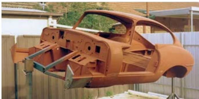
*Alan's E-Type was stripped to a bare shell, chemically treated and primed prior to assembly and painting.*
