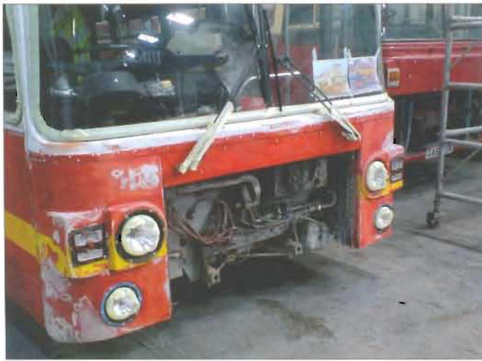
Top left: Fibreglass repairs to front dash. KENNY BARCLAY
