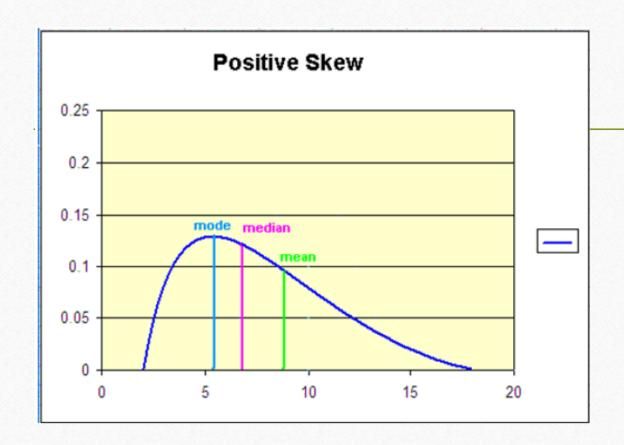
D-) Skewed to the right histogram (positive skewed) / Most of data is shown in the left side of histogram and the tail on the other right side.
