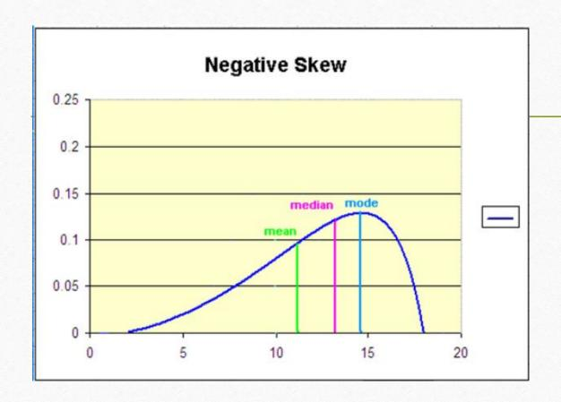
E-) Skewed to the left histogram (negative skewed) / Most of data is shown in the right side of histogram and the tail on the other left side.
