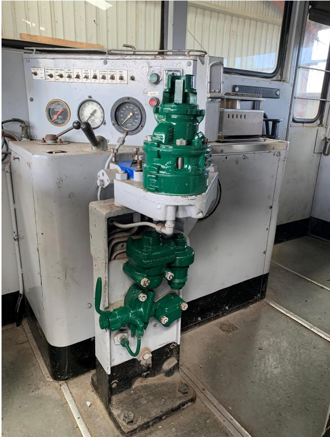
Newly serviced and installed in locomotive 7321 AH7 automatic brake valve, M3 feed valve, isolating valve and equalizing reservoir control valve
