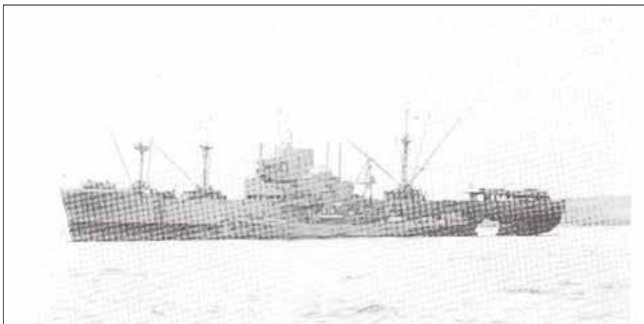
USS Alhena showing torpedo damage. Stern has been raised considerably by shifting oil and armament forward.
