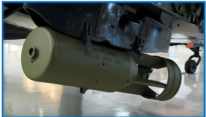
**MK 54 Depth Bomb fixed on an aircraft wing.
