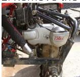
3. Remove the muffler mounting bracket and the eight 8mm bolts that hold the CVT cover on.
