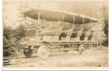
Gas speeder car used on the Cranberry Lake RR between Benson Mines and Wanakena. Previously a was a sightseeing bus.
