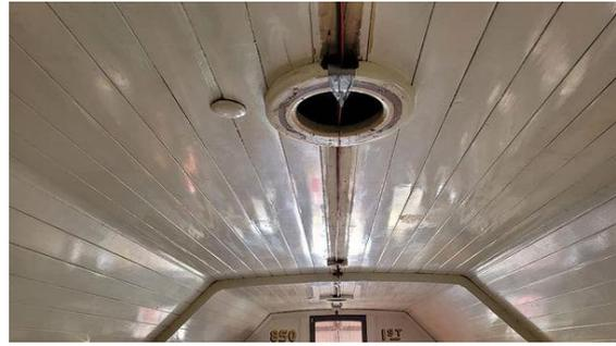
*Interior of CBA850 showing rewiring in progress and installation of LED lighting to take place. Old wiring proved to be inadequate and dangerous.*
