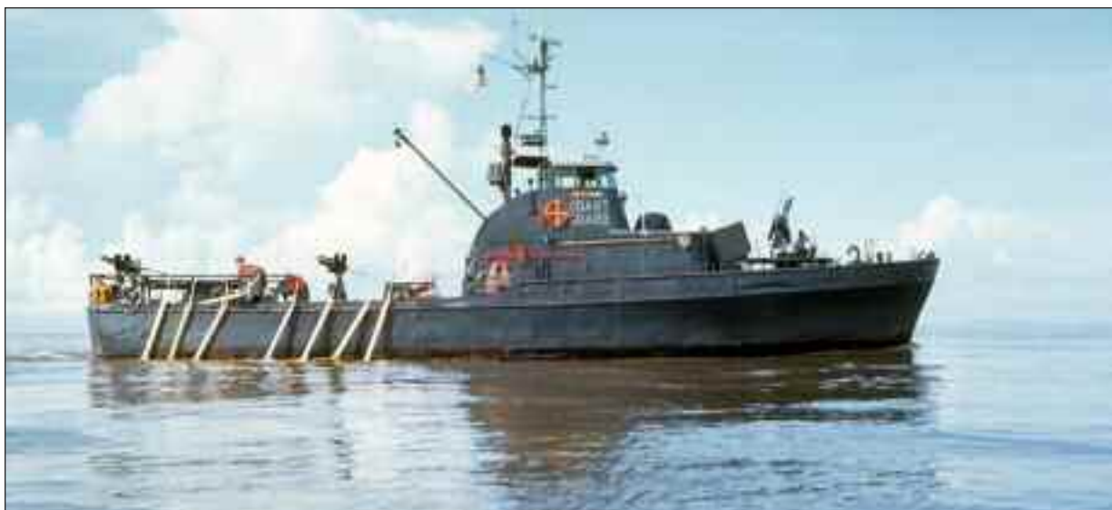
Profile view of Point Cypress showing 50-caliber machine guns mounted on the fantail and amidships with 81mm mortar/50-caliber combination mounted on the bow. (Courtesy of Gordon M. Gillies)
