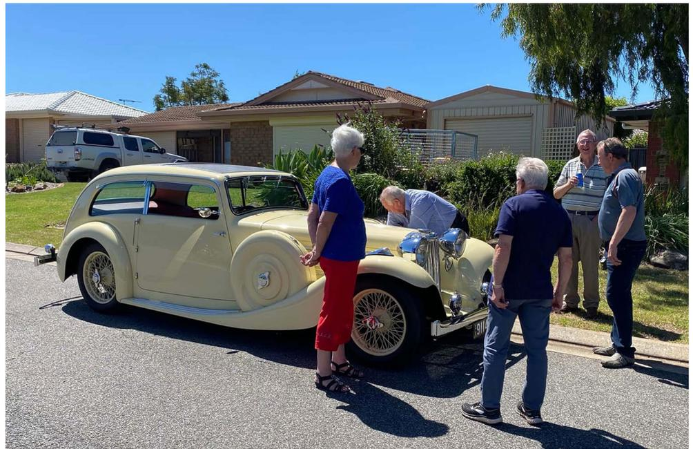
*Malcolm arrived in his Airline. The car was overheating (so was Malcolm!). After an inspection they found that the thermostat was closed in winter position. Electric fan to be installed (that's Bruce Fletcher under the bonnet).*
