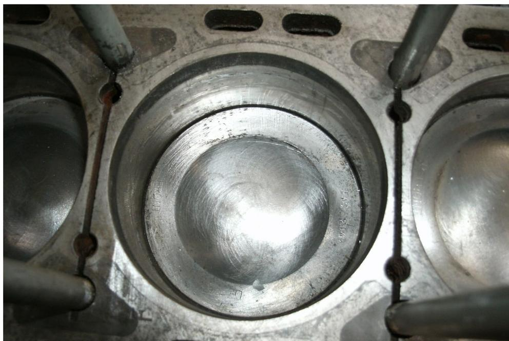
*The temperature differential between the inlet and exhaust side of the block was solved in 1981 by machining longitudinal slots across the block allowing coolant to be able to circulate from the exhaust to the inlet side between the liners, equalising the temperature in this weak area.*
