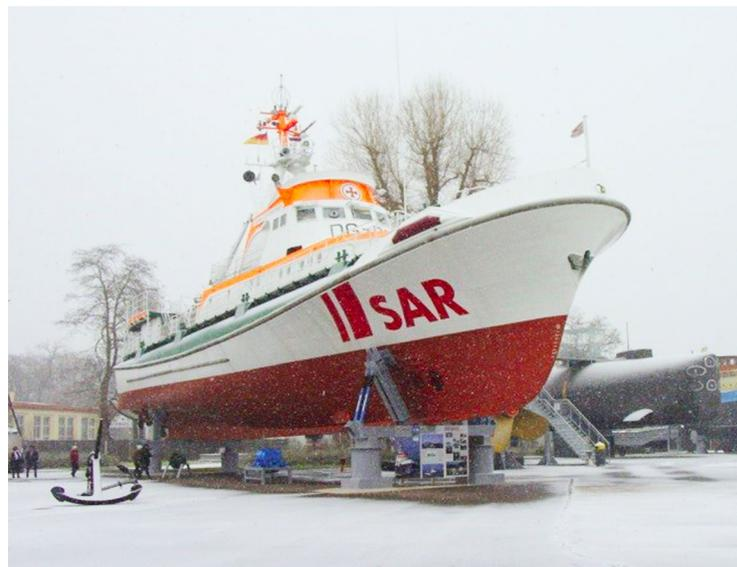
It was a Rescue ship built in 1975 and was the first ship of the large 44 meters class of the DGzRS at the Schweers shipyard. It is powered by three engines with a combined output of 7200 hp and reaches a maximum speed of 26 knots (approx. 48 km/h). The rescue ship is equipped with a small autonomous rescue ship, an on-board hospital, a water cannon for fire-fighting, and many other features.
