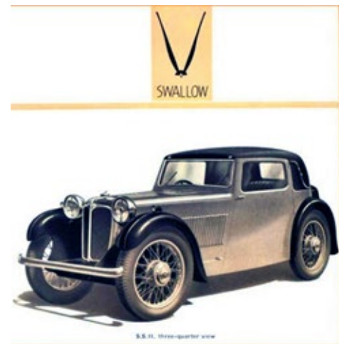
Illustration of a S.S.II. Series 2 with its cycle type wings and carriage top with false irons. Original photographs of the early S.S.II.'s Series 1 are virtually non-existent.
