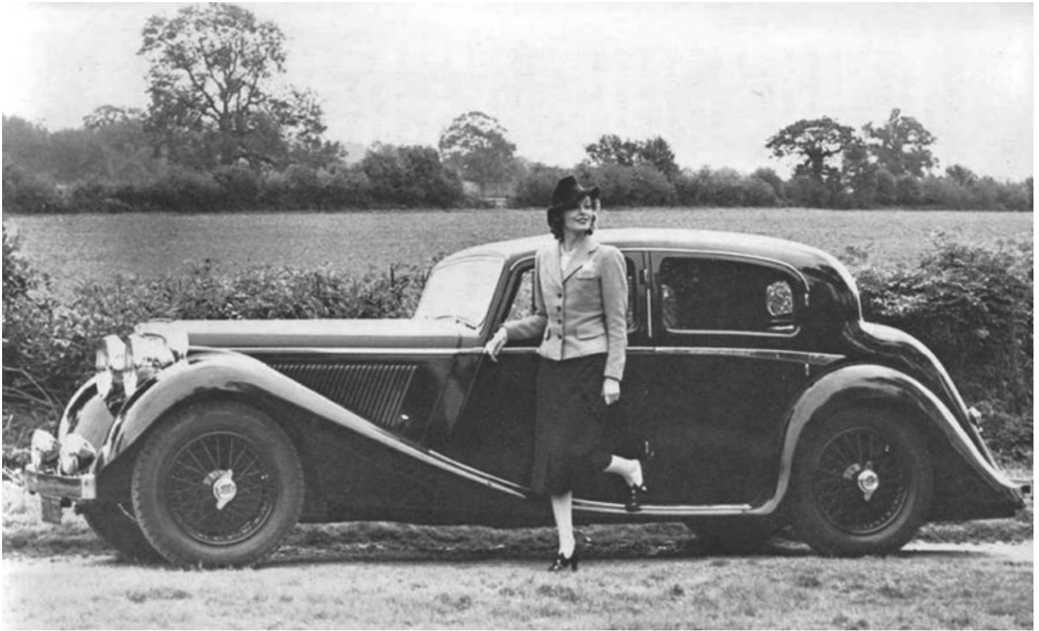
The cars produced in 1938 had an all steel body which was a breakaway from traditional coachwork of steel panels on an ash frame.
