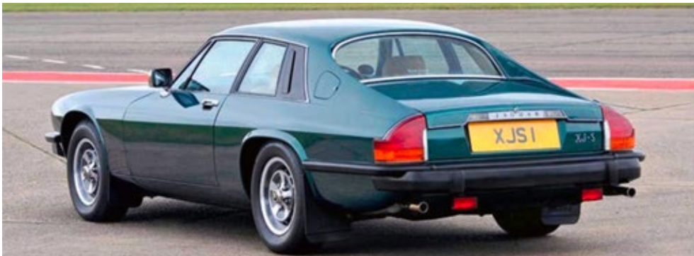
The buttresses on the XJ-S weren't just there for the sake of design but aided aerodynamics and improved stability at high speed by controlling the airflow towards the rear of the car.
