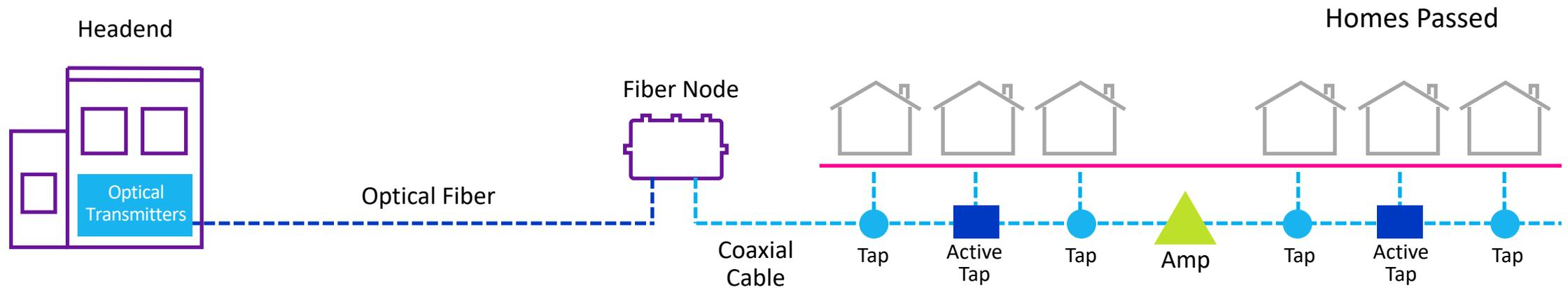
Active Taps would have Amplifiers integrated to boost signal strength... Especially at high frequencies
