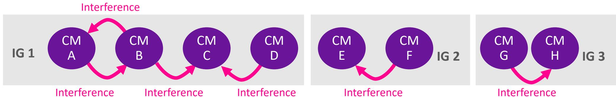
The Transmission Group (TG) is a MAC-level concept... It is the logical merging of one or more Interference Groups to create a larger group of modems that can be treated as a single managed entity on the HFC plant
