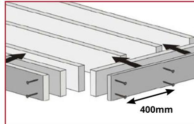
Fascia boards need to be fixed at installed on 400mm centres to prevent warping or buckling. All fascias need to use two screws 40mm away from the ends regardless of the thickness.
