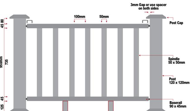
*Note: Portland hand rail is only suitable for installation to a maximum of 600mm above ground level.*
