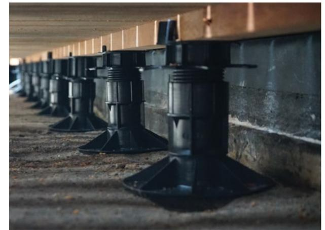
Pedestals offer great flexibility for installation and can be used for decking and paving. They are especially helpful where the installation is close to ground level, pedestals can be used for build ups from 17mm up to 1000mm.
