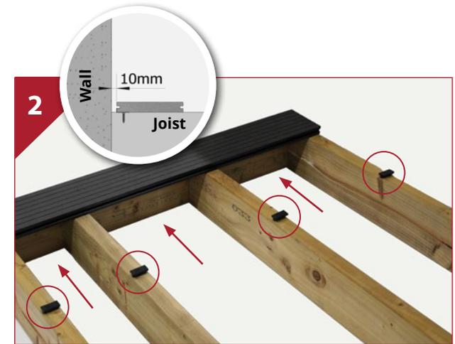
Insert a standard clip into each deck board in line with joist and screw fully but do not over tighten.
