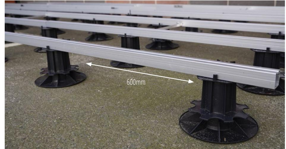
Spacing depends on joist strengths. 600mm spacing shown is for Whiteriver 38mm Aluminium Joists.
