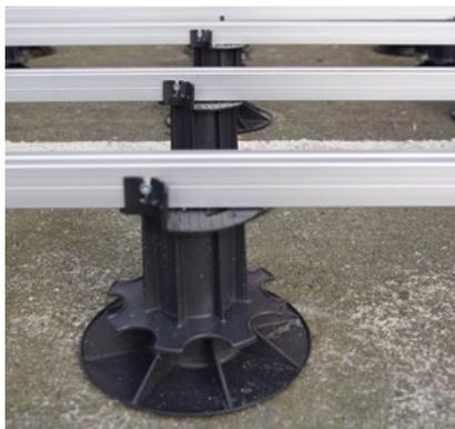
**Step 1** - Understand the spacing's required for the finished product going on top. For composite decking in residential setting using our 38mm aluminium joist, the spacing for the aluminium joist will be 400mm centres and the pedestal spacing will be 600mm.
