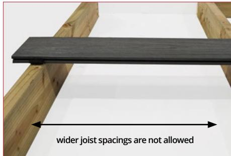
Joists must be set to a maximum of 400mm centres for Portland (350mm Ultrashield). This is to ensure stability and also to avoid warping and cracking of the deck boards.
