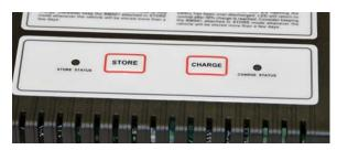
The photo above shows the two operation buttons, and their corresponding LED indicators.
