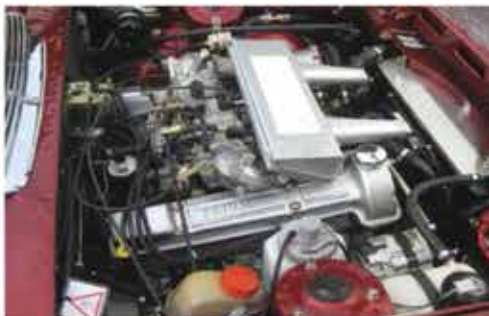
The engine bay looks 'normal' - note alternator in place of PSP and the coolant header tank
