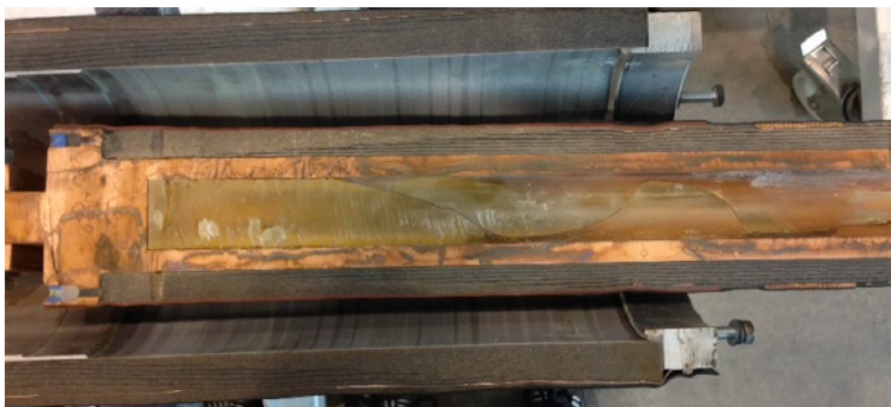
Fig.14: 180-degree cut out of connection tube and bus bar
