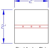
Steel Anchor Plate (2"x2"x3/16" Stl. Angle) Sealed in Fiberglass
