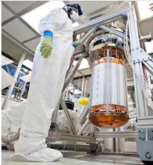
The LUX detector, seen here during the assembly process, relies on photomultiplier tubes that can detect photons emitted during collisions between dark matter and xenon nuclei. MATTHEW KAPUST/SURF
