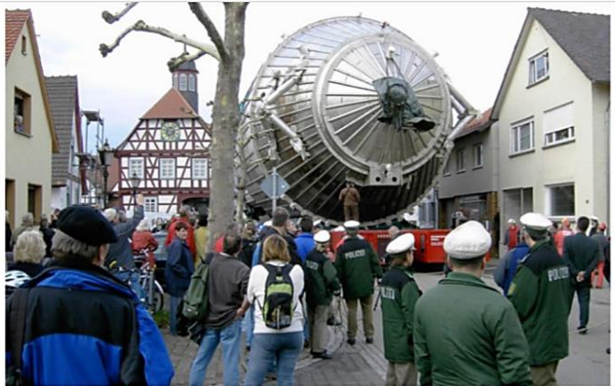
Riding atop a large transport vehicle, KATRIN's enormous 200-ton spectrometer makes its way through the narrow streets of the German village Leopoldshafen in late 2006. Altogether, this essential component of the neutrino-hunting experiment traveled some 5,600 miles (9,000 km) over the course of more than 60 days to reach its final destination at nearby Karlsruhe Research Center. KARLSRUHE TRITIUM NEUTRINO EXPERIMENT
