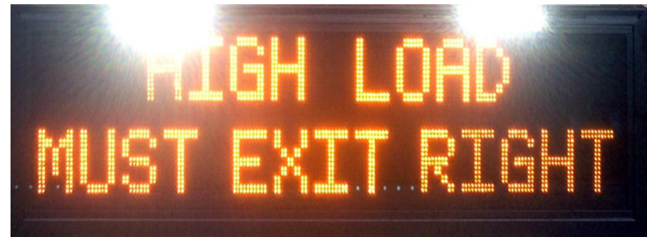
Over Height Sign with Flashing Strobe's
