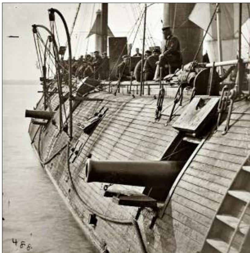
Matthew Brady photograph of the ironclad Galena after the Battle of Drewry's Bluff. A plugged shot hole is visible a little abaft the nearer 11-inch Dahlgren smoothbore, close to the waterline.
