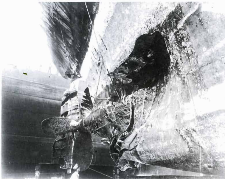
Sailors survey torpedo damage to Cavalier's starboard side aft at Pearl Harbor. Cavalier had been towed nearly 5,500 miles after being hit off Manila Bay.
