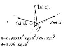
It should be mentioned that the still used "flywheel effect  $WR^2$ " (kp.m<sup>2</sup>) is exactly four times as big as the inertia moment (kg.m<sup>2</sup>) i.e.  $1kg.m^2$  corresponds to  $4kp.m^2$ .
