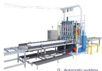
D - Automatic welding and assembling plant for spatial panels
