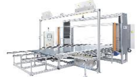
B - Electronic system cutting line by hot wires
