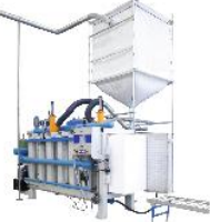
N - Horizontal mold of polystyrene blocks
