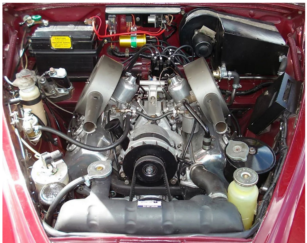
Engine bay of the updated 1967-1969 Daimler V8-250 fitted with an alternator instead of a generator and twin air cleaners, one for each carburettor.
