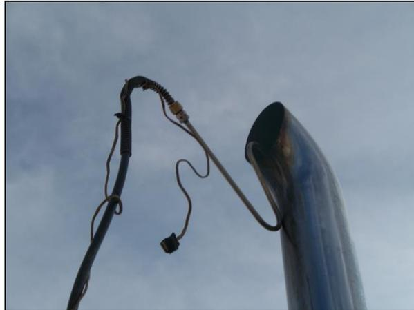
While the emission-sampling probe is in place, and data is being collected, exhaust temperature and pressure are monitored throughout the entirety of the Carbon Balance procedure. The above photograph shows the typical location of the exhaust emissions sampling probe.
