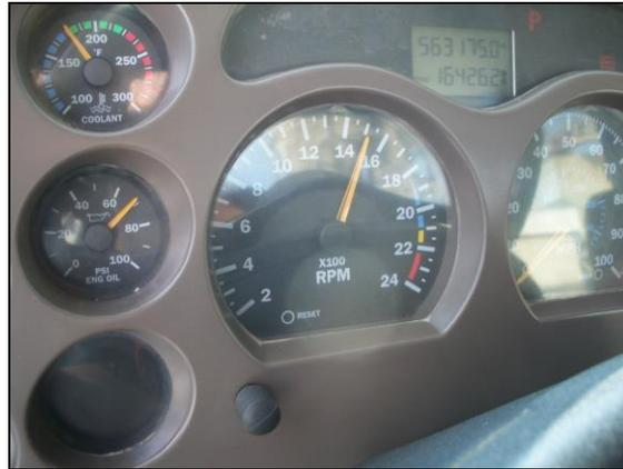
Once engine fluid levels have reached normal operating conditions the Carbon Balance study may begin. The above photograph shows that the engine RPM is locked in place at 1500 RPM. It should be noted that any deviation in RPM, temperature, either fluid or exhaust, would cause this unit to be eliminated from the evaluation due to mechanical inconsistencies.
