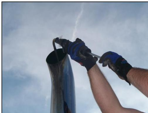
The above photograph demonstrates a typical method in which soot particulate volume is monitored during the Carbon Balance test. This method is the Bacharach Smoke Spot test. It is extremely accurate, portable, and repeatable. It is a valuable tool in smoke spot testing when comparing baseline (untreated) exhaust to catalyst treated exhaust.
