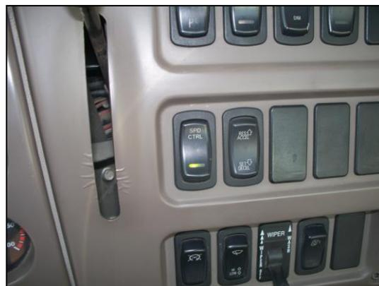
The factory equipped cruise control is utilized, as one method, to secure engine RPM. This provides a steady state condition in which consistent data can be
