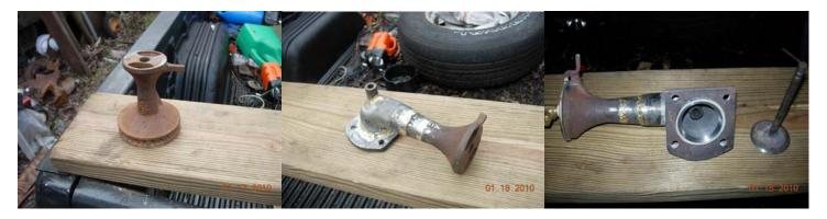
Looking in my junk pile I found a gas burner from an old water heater. I cut one end off to make the fuel mixer from and brazed it to the intake valve assembly. Next I cut the valve seat.
