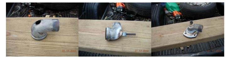
Next you see the hole cut for the valve guide. The valve guide was made from a piece of ½ inch round stock. I used a Chevy small block intake valve I had laying around to center everything up before brazing it together. The next picture is the plate brazed to the intake assembly. I could have used nickel welding rods to do this, but because this part doesn't get hot I chose to braze it as the brass weld looks cleaner and files much easier.
