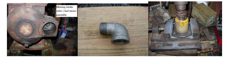
Here is a picture of the place the missing part went. Second picture is the elbow I will use for the intake port and valve seat. Third picture is making a plate to bolt to the engine and weld the intake to. This will make more sense as we progress.
