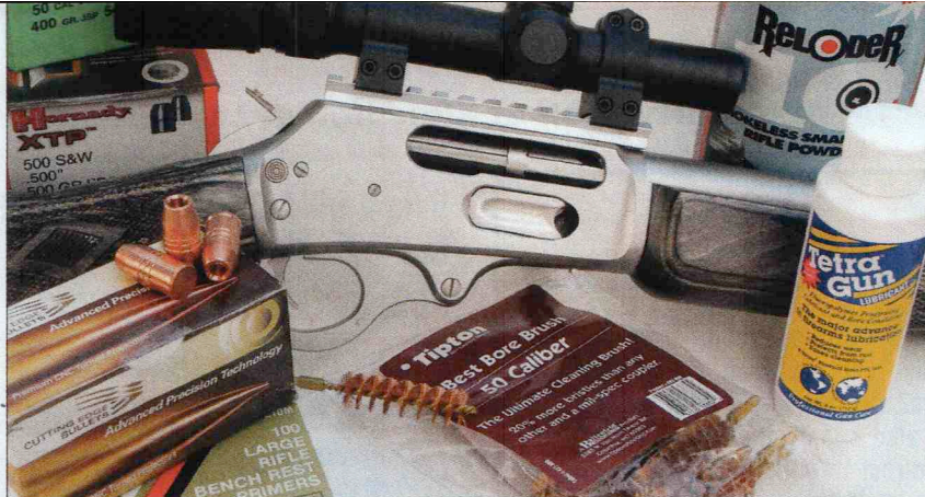
In addition to installing the open sights, T'SOB scope mount, and McGowan barrel, SSK Industries made several modifications to the author's Marlin action, including lengthening the loading port and tweaking several internal parts for reliable cartridge feeding.
