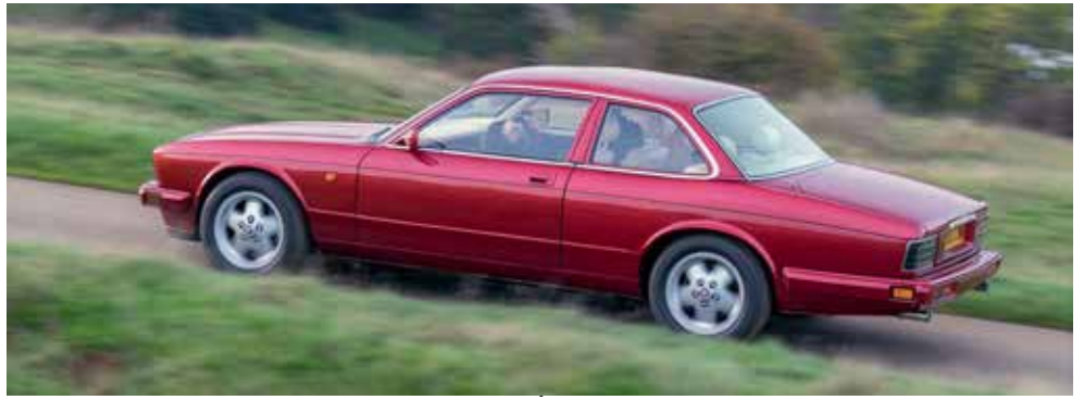
A one-off two-door XJ40 prototype, based on the V12, was built by Jaguar's Special Vehicle Operations Department in Coventry using a shortened XJ40 platform.
