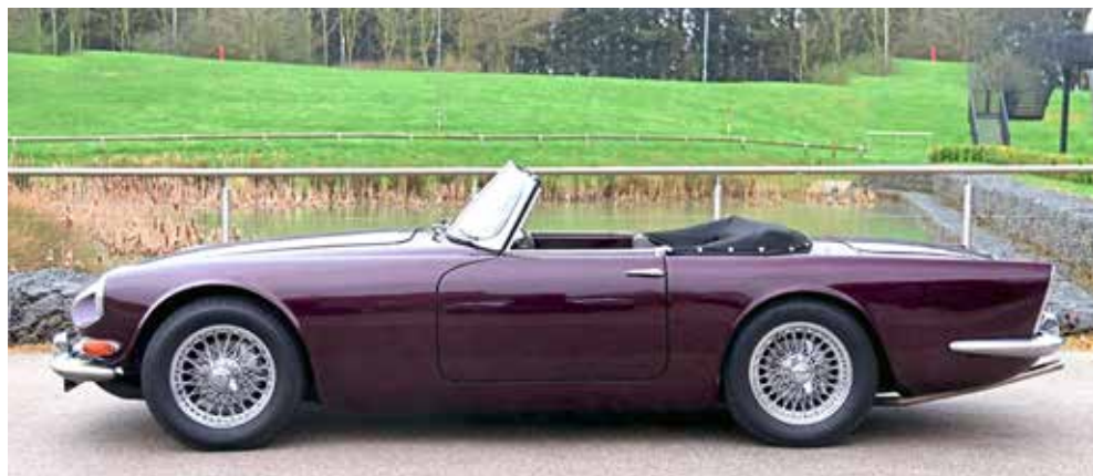
The SP252 prototype was designed and conceived by Sir William Lyons as a replacement for the SP250. A viability study found that the manufacture of the fibreglass body took 2½ times as many man-days to build as the Jaguar E-type, and so the project was shelved.
