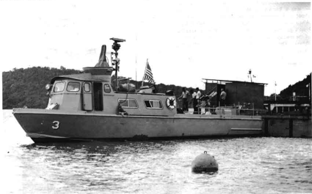
Navy PCF-3 moored at An Thoi in the Gulf of Thailand. Aluminum-hulled 50-foot "Swifts" were manned by a crew of six — one officer and five enlisted men.
