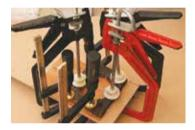
One thing I learnt the hard way was to put enough clamps on, as the first time I tried the veneer was bubbled up and I had to start again. It is important that it is clamped tight, veneer is about 1mm thick so the PVA adhesive soaks in and it wrinkles up like paper. On the instrument panel alone I had 8 clamps, some borrowed from neighbours.
