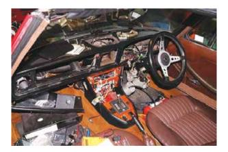
Once the veneer was stuck I gave it 1 coat of a spray can wood varnish so as I cut out the instrument holes etc the wood was less likely to split (You Tube advice). The finishing and light sanding between coats took weeks but I am very happy with it now it is all done.
