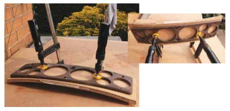
The first thing I made was a former / jig for the instrument panel. This was made from BENDI MDF (a UK brand name), glued 2 pieces back to back with PVA glue and clamped them to the instrument panel, once this had dried I had my former, which I have to say works really well. I did the same for the
