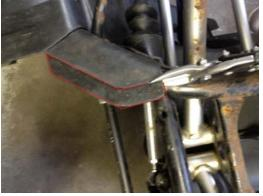
3. On each lower panel measure in 1.5" from the inner edge and then draw a line. This strip then needs trimmed off of each lower side panel. Section outlined in red as shown below needs removed.
