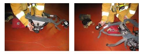
Push in and turn cylinder valve counter-clockwise, fully open. Compare pressure on remote gauge to pressure on cylinder.
