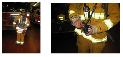
Push inward and close cylinder valve. Bleed residual pressure using the purge valve.
