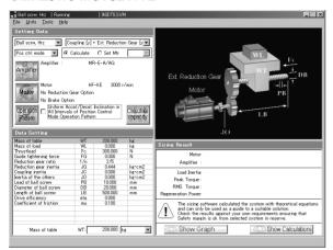
A user-friendly design facilitates selecting the optimum servo amplifier, servo motor (including the servo motor with an electromagnetic brake) and optional regeneration unit just by entering constants and an operation pattern into machine-specific windows.
