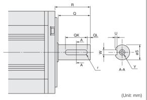
Notes: 1. The motors with the keyway shaft (with/without key) and the D-cut shaft cannot be used in frequent start/stop applications. Loose keys may damage the motor shaft.
