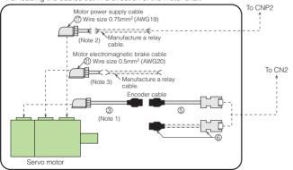
• For leading the cables out in an opposite direction of the motor shaft
