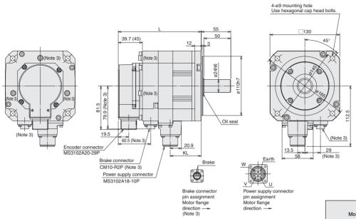
Variable dimensions KL 120 (154.5) HF-SE52(B)JW1-S100 57.8 HF-SE102(B)JW1-S100 142 (176.5) 79.8 164 (198.5) HF-SE152(B)JW1-S100 101.8
