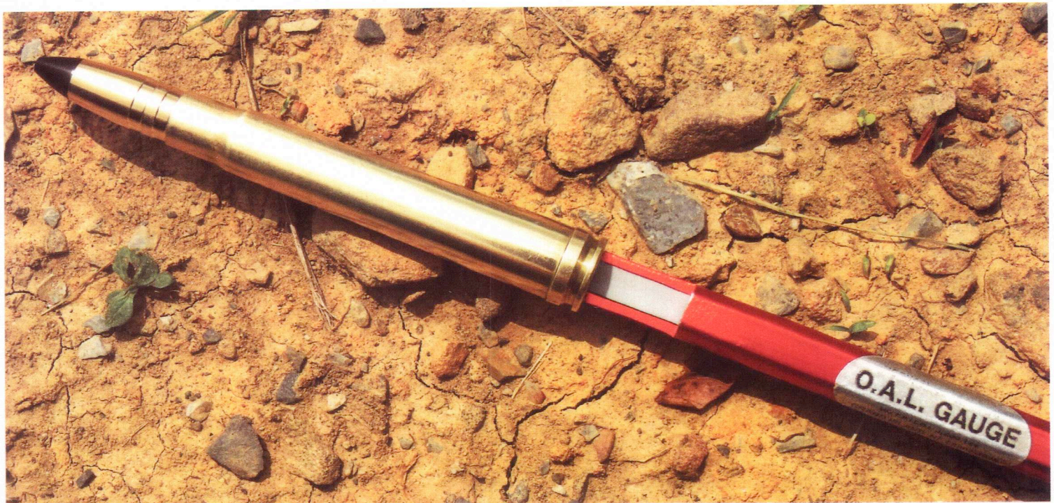
Hornady's L-N-L O.A.L. Gauge helps to determine length to touch rifling with a given bullet
