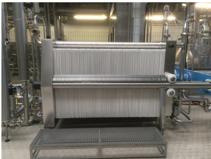
A typical plate filtering machine. The chilled liquid is passed through the many plates (filters) under pressure.
