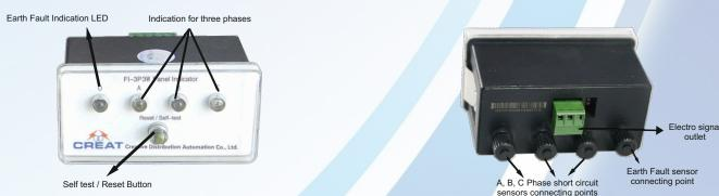
The panel fault indicator can be installed on the enclosure of the switchgear and it connects with the sensors via a fiber optic cable.
