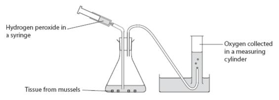
Describe how this apparatus could be used to compare the catalase activity in two different types of mussel.
