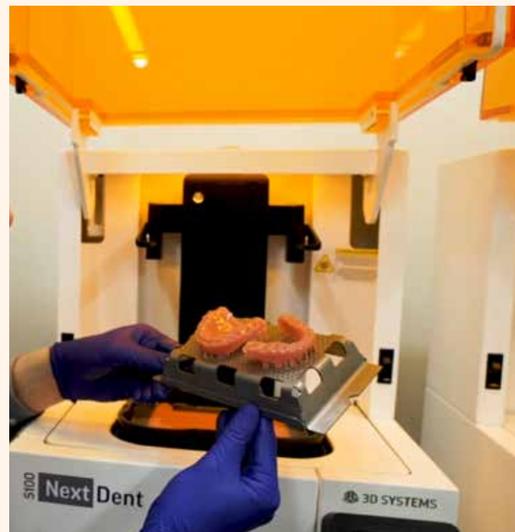
3D Printed Denture base using NextDent™ biocompatible material using NextDent™ 5100
