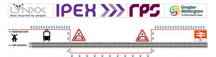
The second scheme shows an alternative approach. In this, the high cost of rebuilding one bridge is justified because it enables the OLE to be run all the way to the second bridge, at which point it ends completely, thus saving the cost of any further OLE and buried cable. This approach is only viable if the trains have sufficient battery autonomy to run the twice the length of the gap (there and back) and run their auxiliary loads for the whole time, including the station dwell time.
