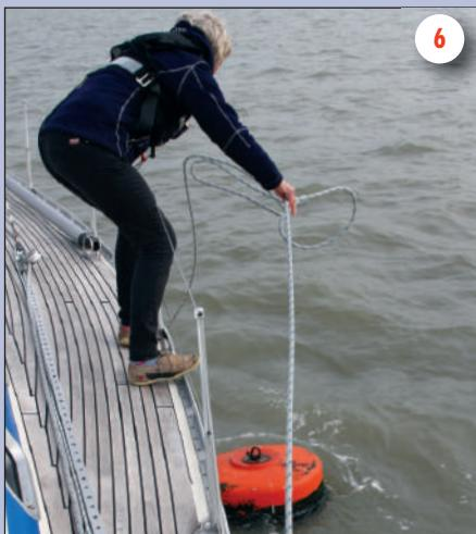
There are devices for threading lines through hoops, round bars and shackles and if you can't reach down to the buoy you may need to use one of these. Remember to use a rope for the lasso that sinks and allow the rope to drop below the buoy so it catches on the chain, otherwise it can easily flip off.
