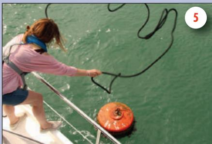
Or you can secure the running end on the winch and with plenty of slack in the line and four coils, lasso the buoy (6). Again the boat will be pushed back by the tide and the buoy will end up at the bow. You then need to attach a line to the buoy from a cleat on board.
