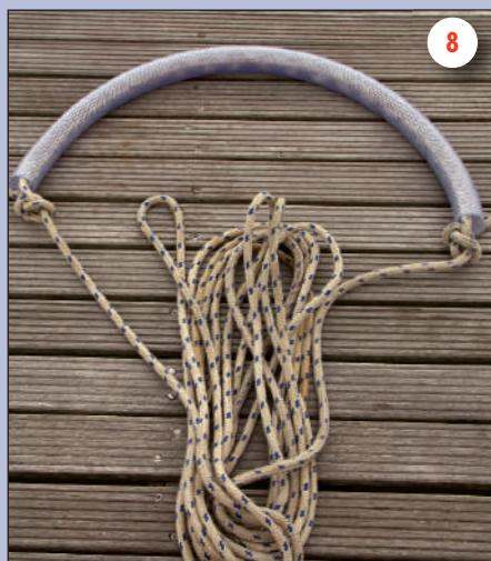
A heavy-duty line for me is a rope to chain to rope affair with the chain inside a plastic tube (8). With one end of the rope attached to a bow cleat and the buoy alongside I drop the chain over the buoy.
