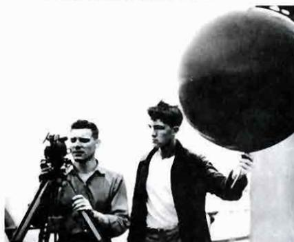
(Left) Checking wind speed and direction. (Right) Launching the weather balloon.
