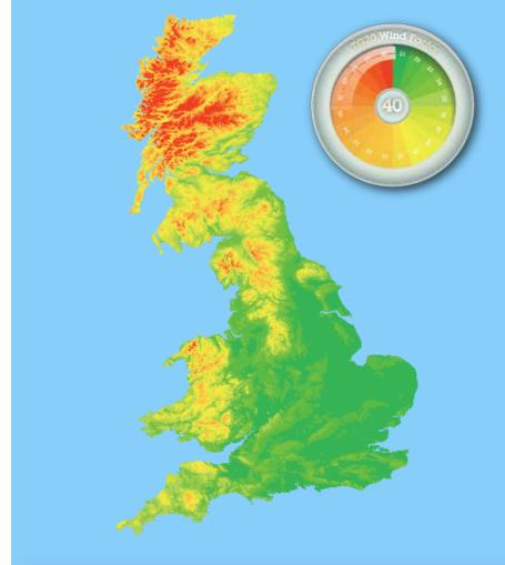
$$\begin{split} S_{wind} &= \max \left\{ dir \mid 0..30..270 \bullet S_{wind,dir} \right\} \\ S_{wind,dir} &= V_{b,map} \times T_{wind,dir} \times \left( 1 + 0.001 \cdot A \left( \frac{10}{\max(z,10)} \right)^{0.2} \right) \times C_{season} \times C_{dir} \times \sqrt{\frac{C_{\epsilon}(z).C_{e,T}}{C_{\epsilon}(z).C_{e,T} max}} \end{split}$$
