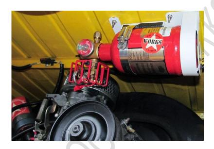
The fire suppression system is fully active once located in the engine bay. For added security and peace of mind the dashboard LED indicator light should be installed. However, the system is operational without this being installed but as there is a visual indicator every time the ignition is turned on it avoids driving with a non-operational system.
