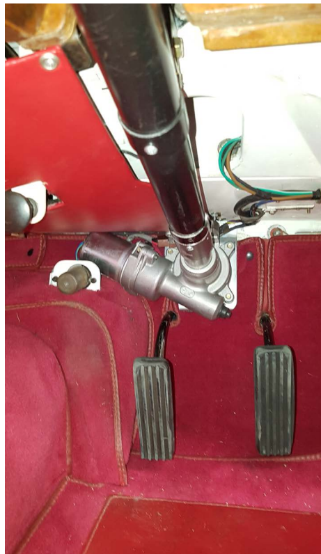
Column installed in XK140
