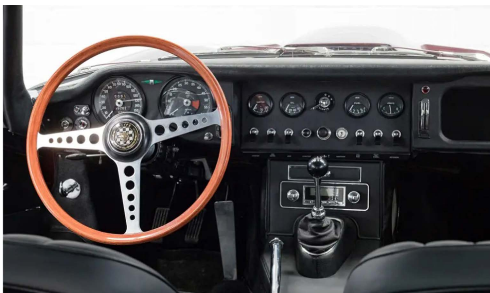
The manual gearbox can be retained to maintain the classic E-Type driving experience. The dashboard is unchanged and the dials and gauges are repurposed.
