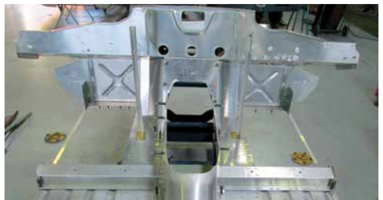
A work of art, not just a car in the making. The correct period rivets were used, and along with specific aluminium sheeting imported from the U.S. They provided a final result to please the most fastidious of inspections.
