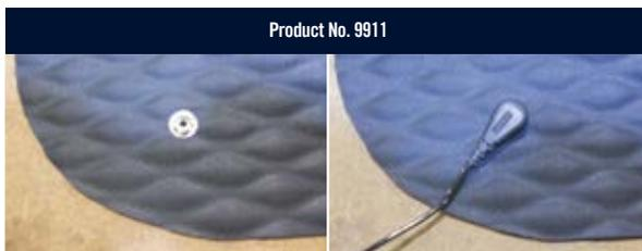
**Heel Grounders** are made for workers wearing rubber soles and other insulating shoes. They allow static electricity to pass around the shoe into the ESD matting. Fasten the Heel Grounder to the heel of the shoe with the Velcro and allow the fabric strip to touch the sock or skin for best performance.
