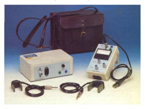
Ideal for pin point location of high resistance faults on floating DC systems
