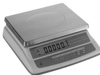
Figure 1.4 Electronic medium top-pan balance, with a capacity of 2100 g and a resolution of 0.01 g (photograph courtesy of ELE International)
