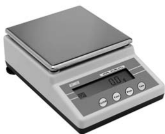
Figure 1.3 Electronic coarse top-pan balance, with a capacity of 30 kg and a resolution of 1 g (photograph courtesy of ELE International)
