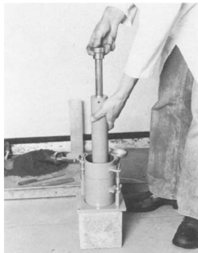
Figure 6.11 Compacting soil into mould
