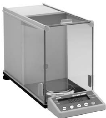
Figure 1.5 Analytical balance, with a capacity of 210 g and a resolution of 0.1 mg (photograph courtesy of ELE International)
