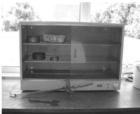
Figure 1.6 Large-capacity electric drying oven (photograph courtesy of Cranfield University)
