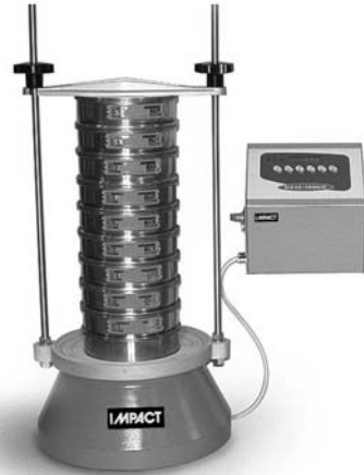
Figure 1.22 Sieve shaker, high frequency vibratory type (photograph courtesy of Impact Test Equipment)
