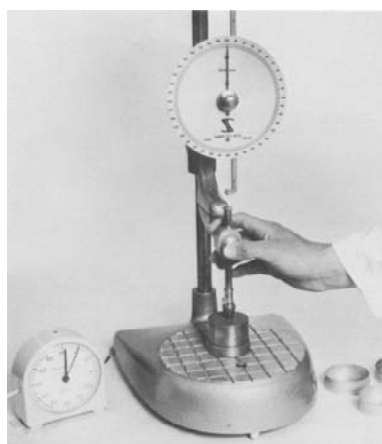
Figure 2.12 Cone penetrometer test immediately after penetration
